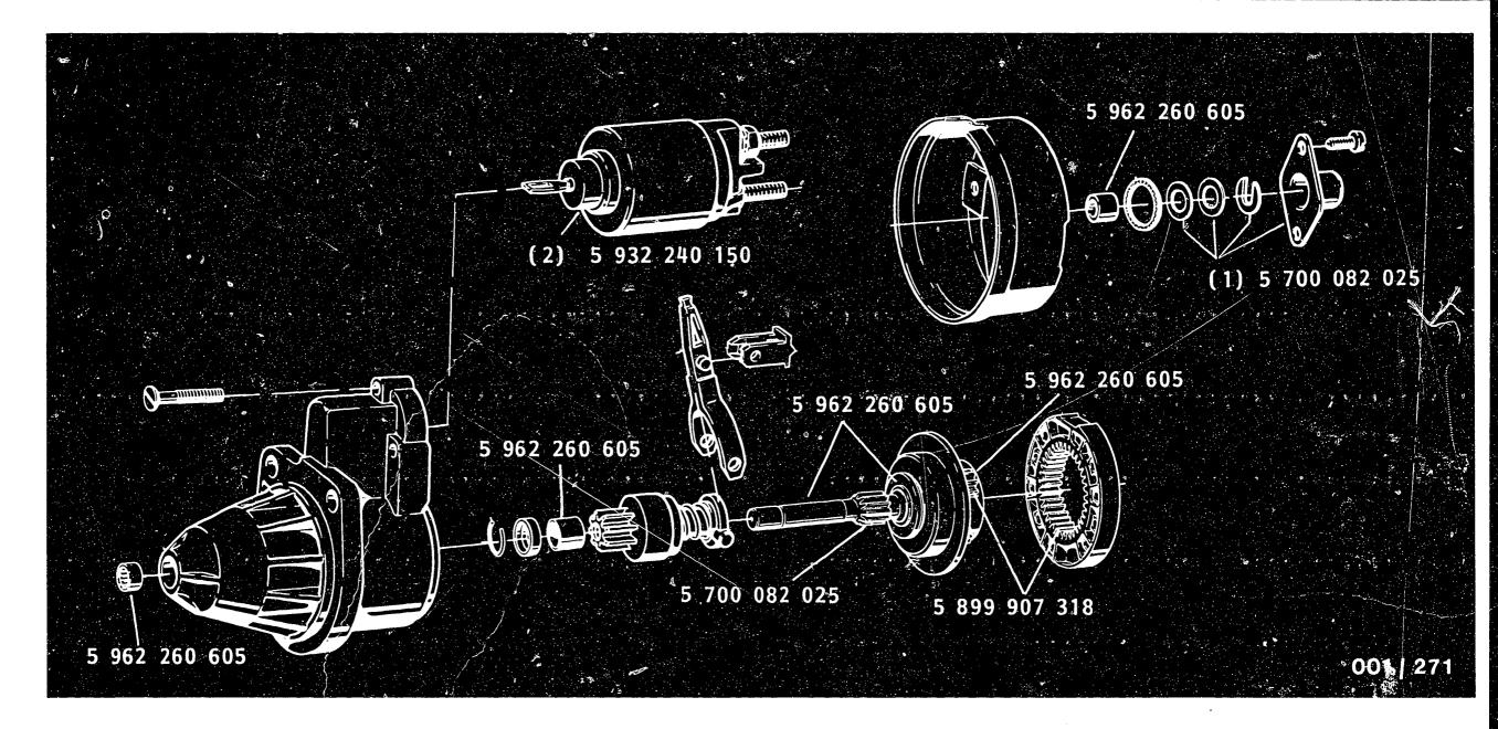
1 = Do not grease the inside of the holding or compensating washers or of the closure cap until after adjustment of the longitudinal play of the armature. Then grease lightly using 5 700 082 025 (approx. 0.2 g).
